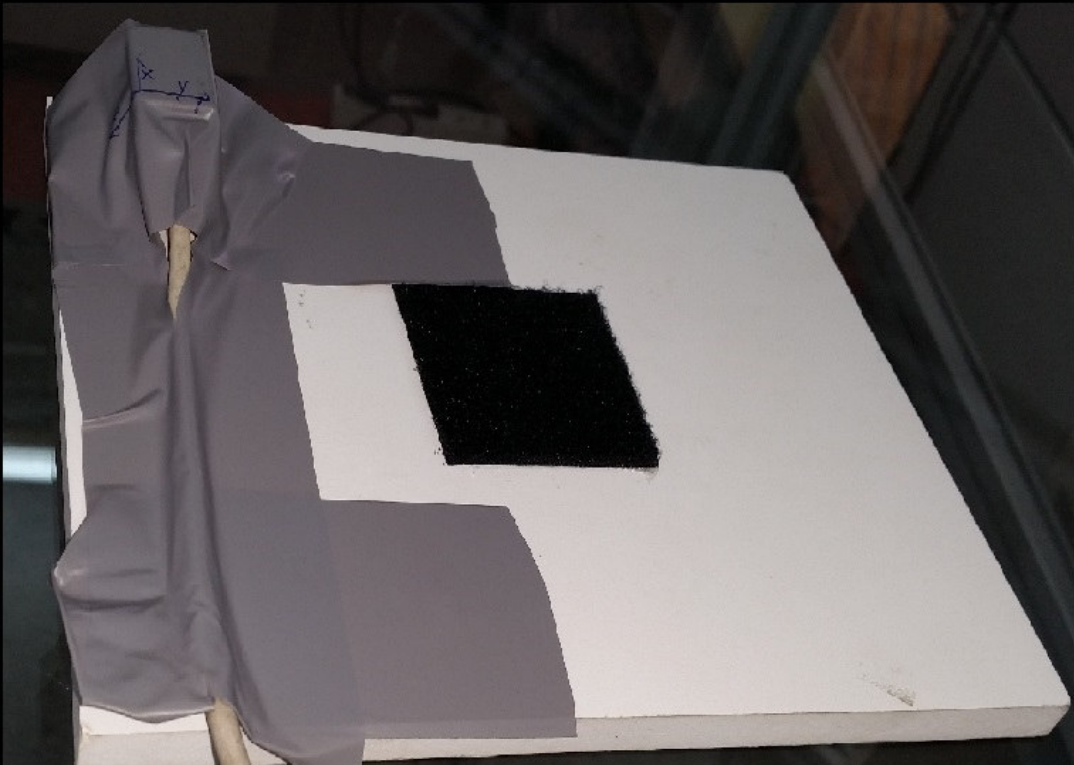
2. Checkerboard for detection in cameraframe ("/camera_left_frame") and FoB tracker in "/tracker_left_raw"
